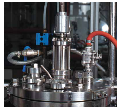
Reactor for the synthesis of absorbable polymers for medical products
