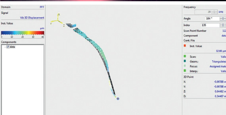
Deflection shape of the PS instrument during ultrasonic activation.
