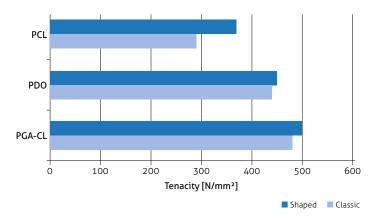
Tenacities are given as the linear tensile strength (LTS) in relation to the effective diameter.
